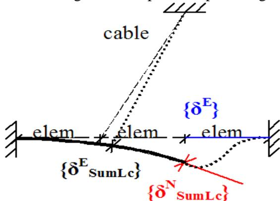
Fig. 4: Automatic kink correction in erection control mode
