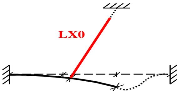
Six input values are needed for defining the stress free fabrication shape of a beam segment as presented in Figure 6. With activating the option "Erection Control", appropriate changing the structural system is done automatically by the software.
