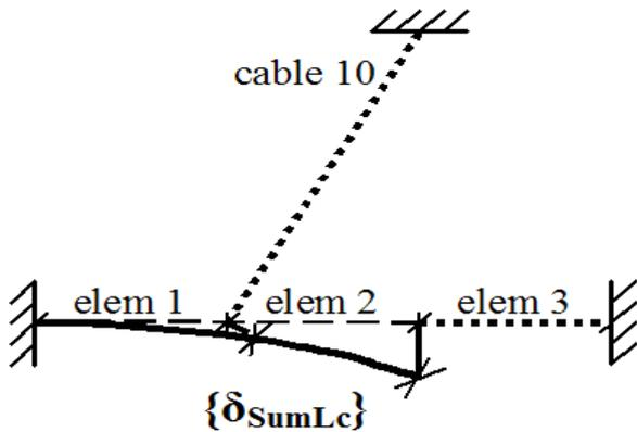
Fig. 3: Missing geometric info when assembling cable 10 and element 3
