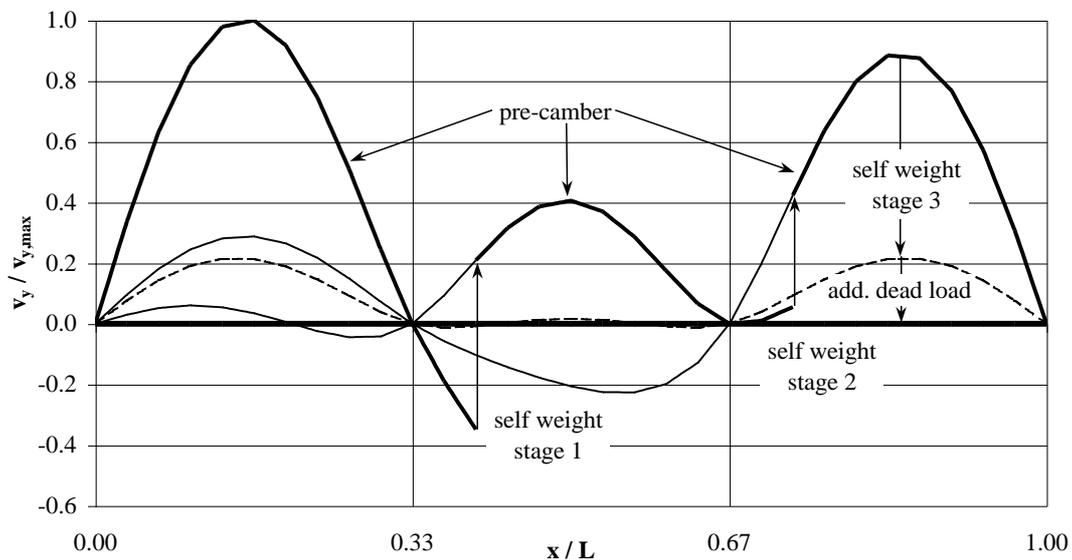
Fig. 2: Pre-camber shapes and displacements during assembly
