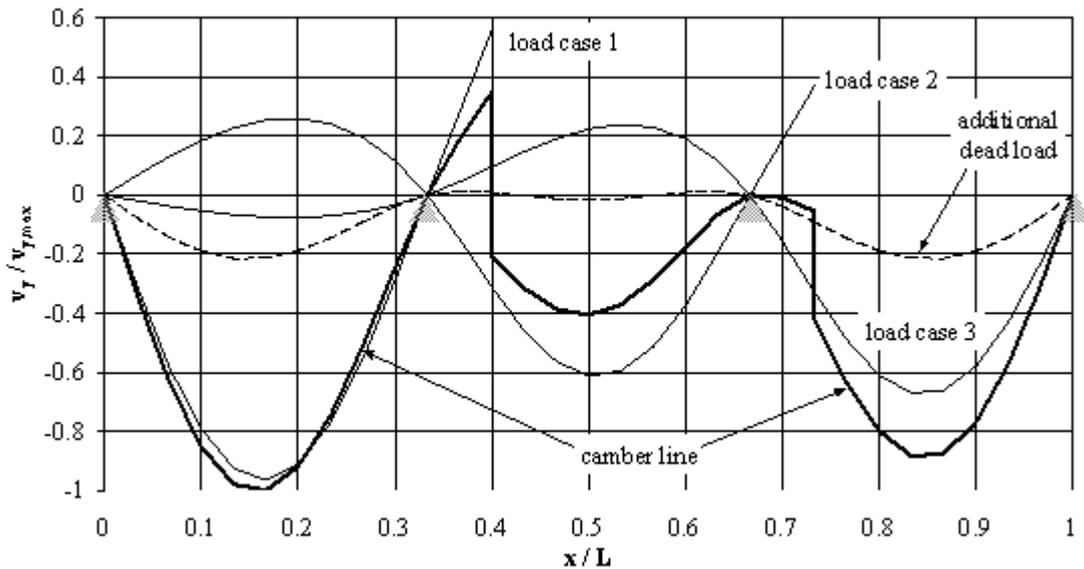
Fig. 1: Deflection lines for a three-span bridge
