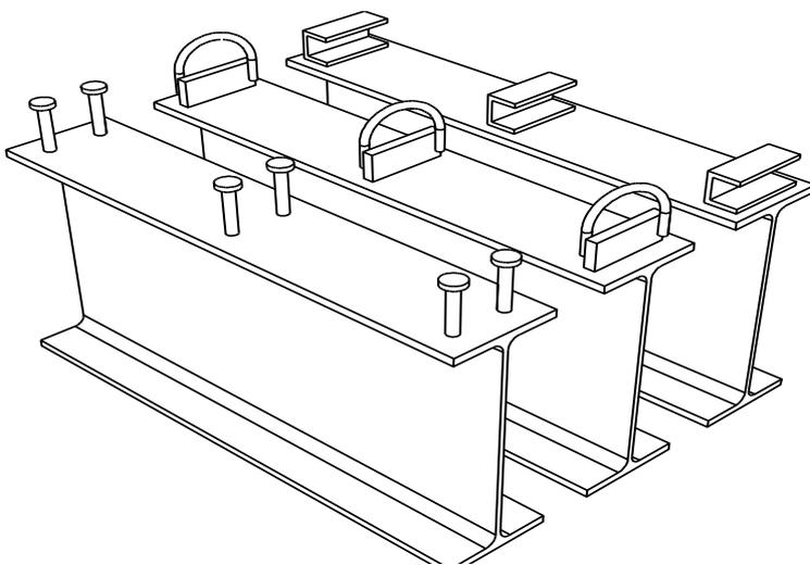
Figure 7 Different types of shear keys
