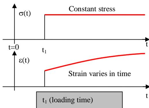
Fig. 3. Creep – development of the creep strain over the time under the constant stress
