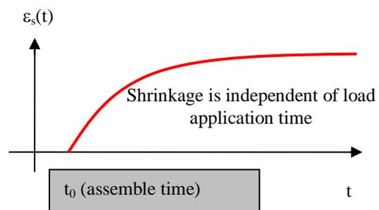
Fig. 4. Shrinkage – development of the shrinkage strain over the time
