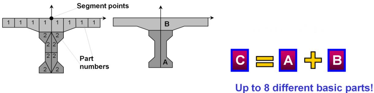
Figure 1 Composite cross-section with cross-section parts
