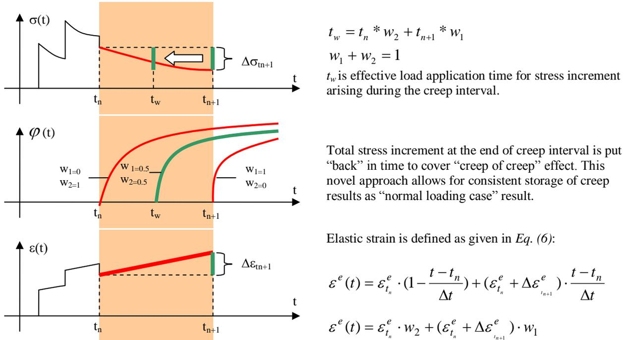
Fig. 6 Stress, creep factor and strain development in the time interval  $t_n$  to  $t_{n+1}$
