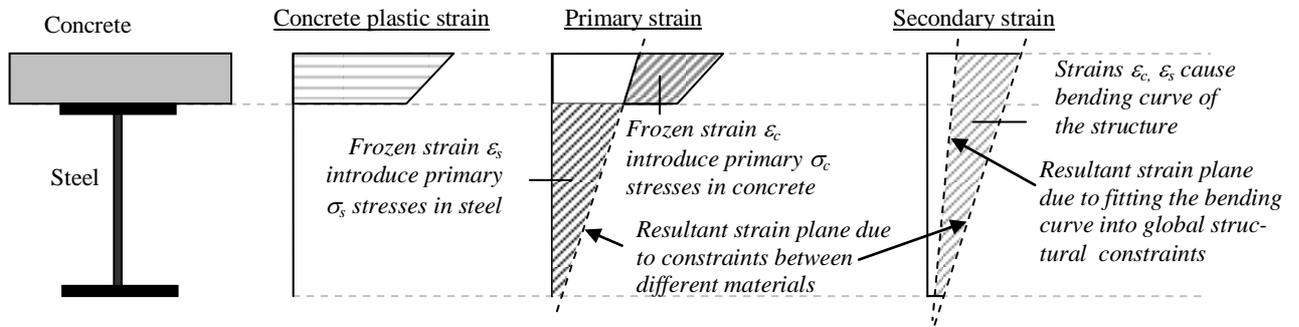
Fig. 5: Stress, creep factor and strain development in the time interval  $t_n$  to  $t_{n+1}$
