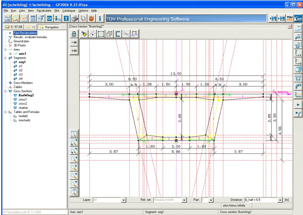
Figure 1: Interactive graphic construction of cross-sections
