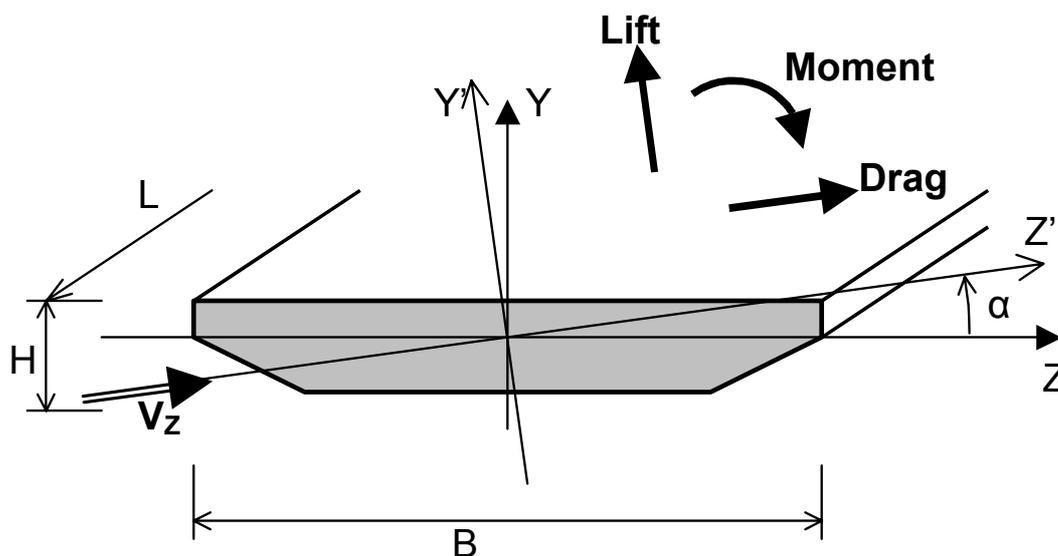
Figure 4: Wind forces acting on the bridge section
