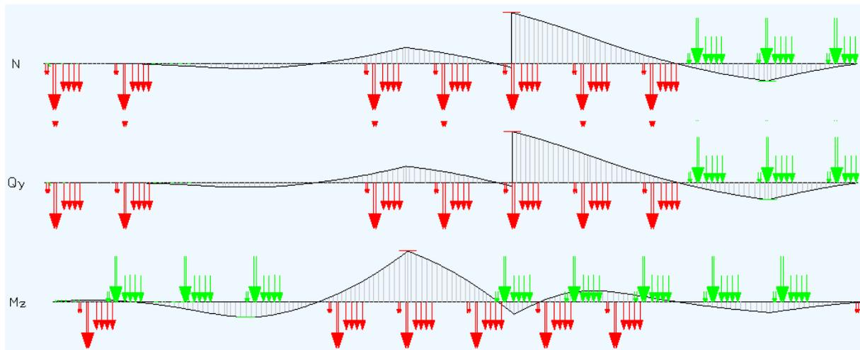
Figure 2: Influence lines and relevant traffic loading in accordance with Indian code
