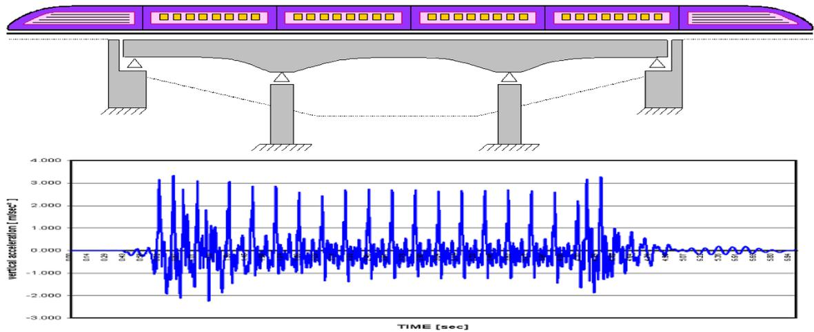
Figure 3: Vertical acceleration time history at mid-span due to a passing train
