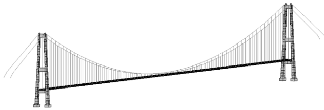
Fig. 13. Structural model of Hardanger bridge.
